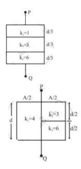
(i) The capacitor in the first diagram is a series combination of three capacitors of plate separations d/3 and plate areas A, with C<sub>1</sub> filled with air ( $k_1$ = 1), C<sub>2</sub> filled with a dielectric of  $k_2$  = 3, and C<sub>3</sub> filled with a dielectric of  $k_3$  = 6.
